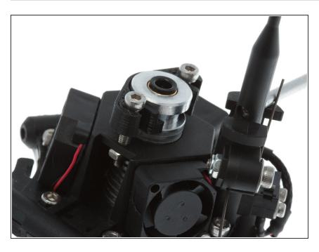
Slide the bottom clamp on. This is the thicker of the two printed pieces.
