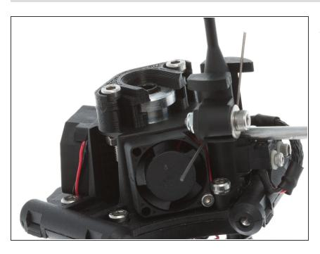
Install the top clamp; pull up on the clamp mounting screws and finger tighten the screws. We'll clamp the K-Head down in place in a minute, but for now we need to make sure that the heat block is oriented correctly in the end effector housing so it doesn't crash into the glass during auto levelling probe retract.
