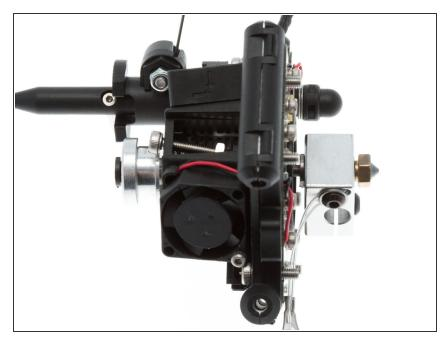
Insert the K-Head from the bottom of the end effector opening, until the bottom of the groove mount is flush with the top edge of the end effector.
