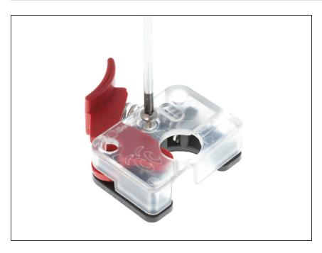
With a #1 Phillips screwdriver, remove the single #1 Phillips drive screw from the SeeMeCNC EzStruder Top.
