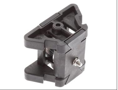
Using one of the Idler Subassembly Top/Bottom that has had an M3 Locknut glued in place, add it to the top of the assembly and tighten the 30mm screw. Ensure that the pulley still spins freely.
