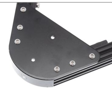
Using M3 x 6mm Button Head Cap Screws (BHCS), install vertex cap plates over the end of each vertex.
