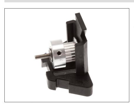
Insert an M3 30mm SHC Screw into the Idler Subassembly Front/Back, then slide a pulley onto it with the thick end facing the narrow side of the Idler Subassembly Top/Bottom.
