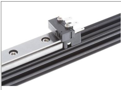
Be extremely careful not to let the carriage slide off the end of the rail. This could result in loss of bearings.
