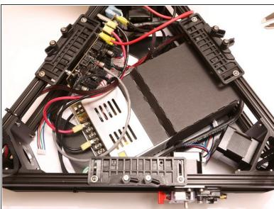
Holding the PSU, flip the lower triangle over and secure the PSU in place with 4x M4 FSC, included in the PSU Kit.
