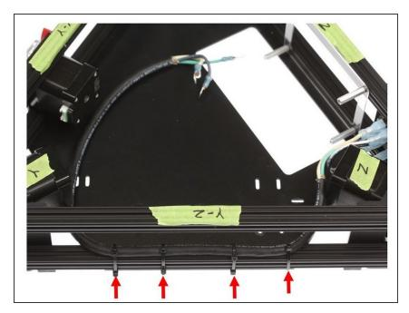
Daisy-chaining the included zip ties, secure the AC wiring bundle to the lower Y-Z OpenBeam extrusion on the printer, looping the zip tie through the oval opening on the power supply mount panel.
