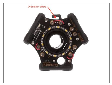
Fan polarity orientation is not laid out the same at each wire-chase hole.
